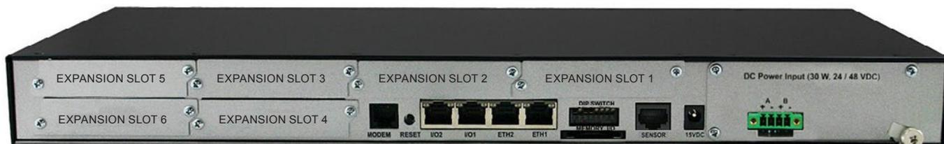
Slot number arrangement (using the SiteBoss 550-6 as an example)
